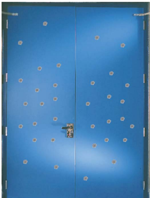
Typical Bullet Resistant Door Profile
