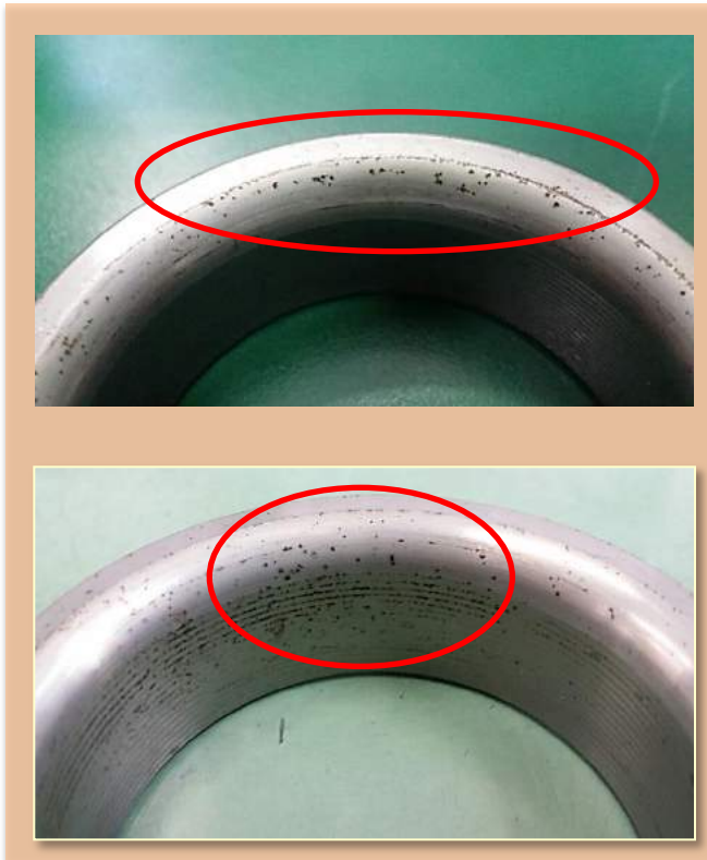
Surface condition Before
